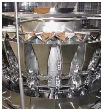
Multi-head weighers for precision dosing of the crispies
