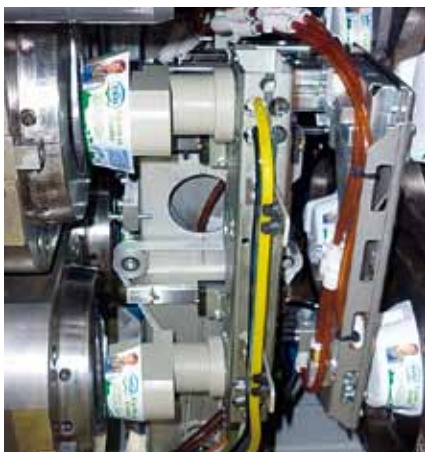
Insertion of the IML label and extraction of the finished twin compartment pot
